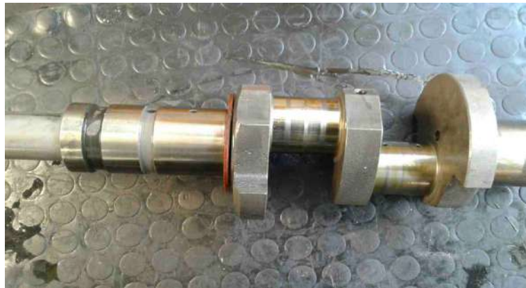
Figure 7. Shaft journals after qualification tests – PAG68.
