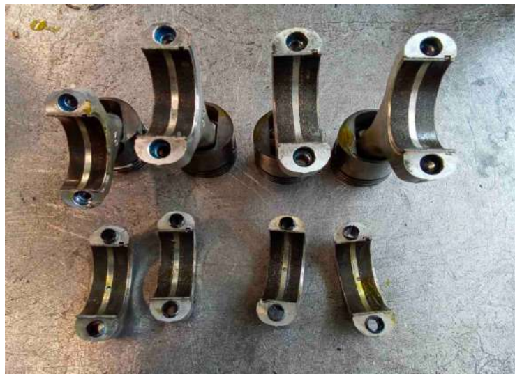
Figure 10. Bearings and pistons after qualification tests – POE85.
