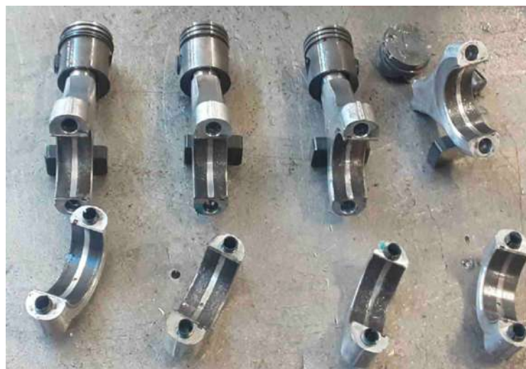
Figure 8. Bearings and pistons after qualification tests – PAG68.
