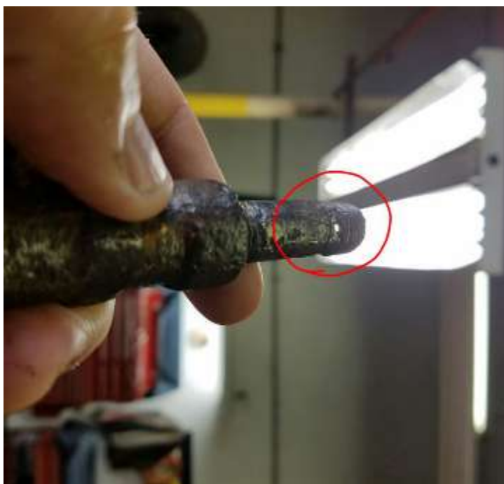
Figure 25. Hole in the ½" Service Valve
