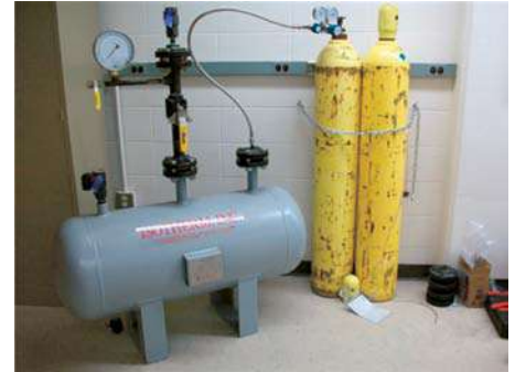
Figure 1: Pressure relief valve test rig (University of Wisconsin-Madison, IRC 2010).
