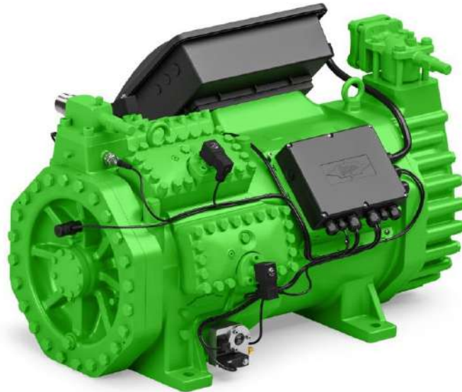
Figure 1. Eight-cylinder CO 2 compressor equipped with built-in intelligent module and wired accessories (capacity control system, oil pressure control, oil level management, discharge gas temperature, oil heater, and motor PTC sensors, not shown).
