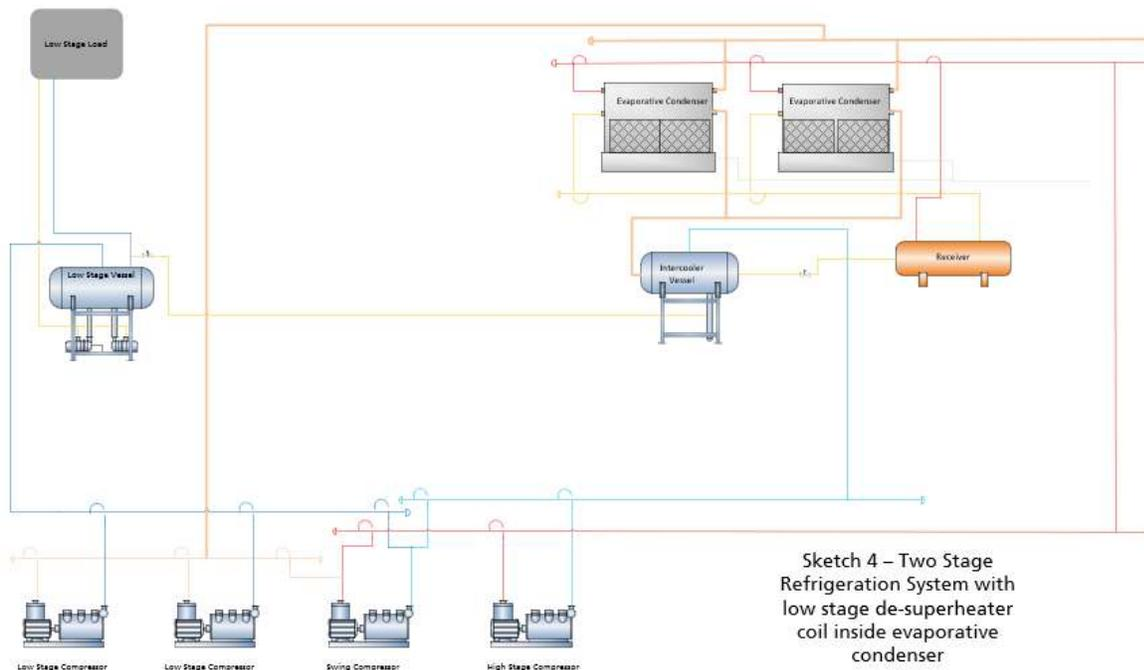
Figure 4. Two-stage refrigeration system with a low-stage de-superheater coil inside the evaporative condenser.
