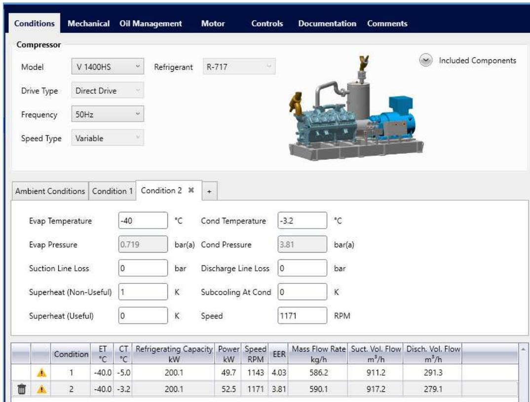
Figure 11. Initial high-stage compressor criteria.
