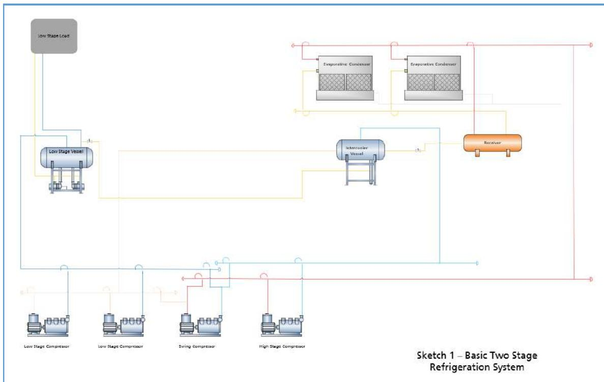
Figure 1. A simple two-stage plant used for low-temperature applications.
