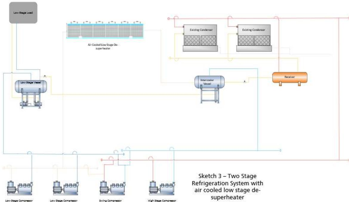
Figure 3. Two-stage refrigeration system with air-cooled low-stage de-superheater.
