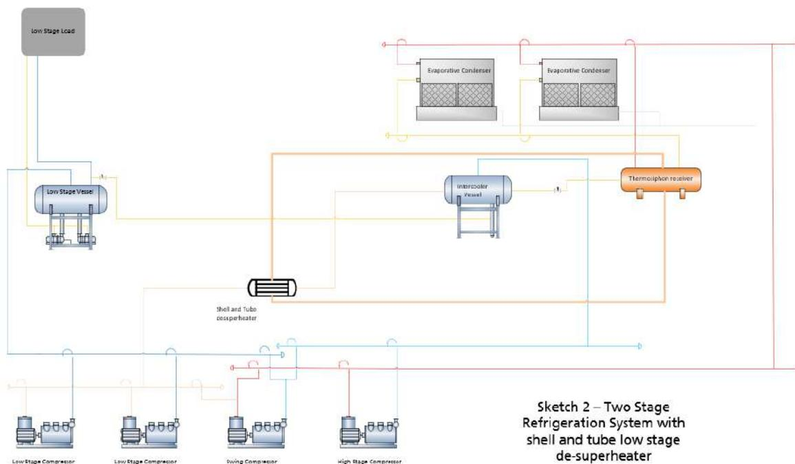
Figure 2. Two-stage refrigeration system with shell-and-tube low-stage de-superheater.
