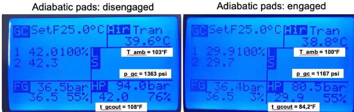
Figure 11. Field measurements with and without adiabatic gas cooler operation.
