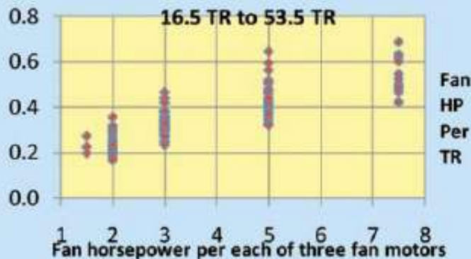
Figura 1 Three Fan CH Evaporators, 4 FPI, 0.0" Static, 10F TD 16.5 TR to 53.5 TR
