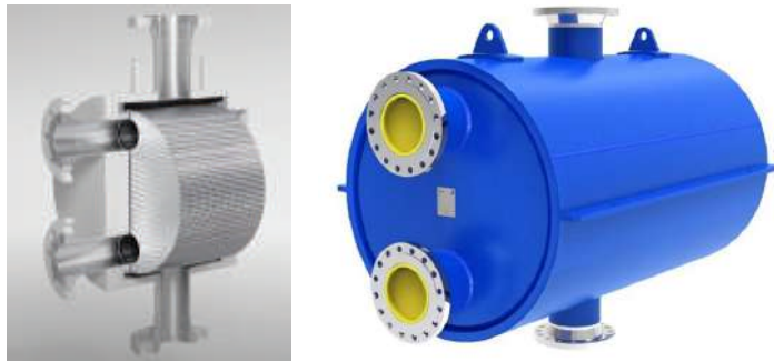
Figure 2. A cut-through view of a plate-and-shell heat exchanger. It offers the high integrity of a fully welded heat exchanger (like shell and tube), but the small footprint and refrigerant charge of a plate heat exchanger.
