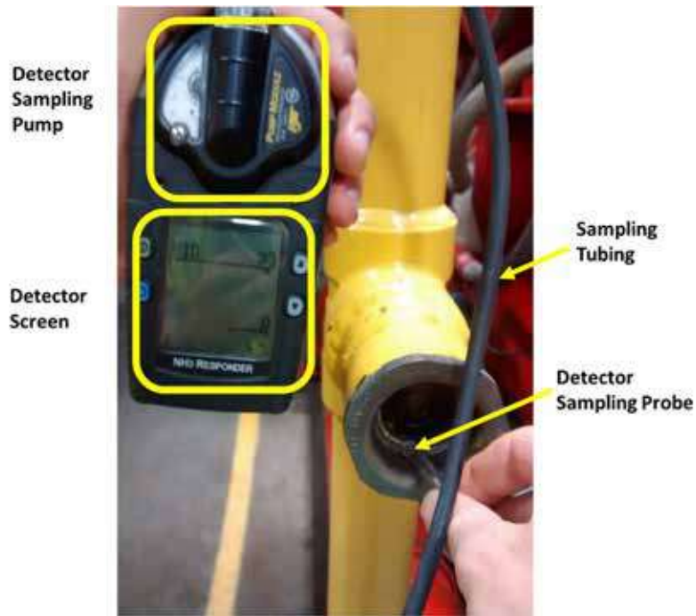
Figure 1. Refrigerant detector equipped with an integral vacuum pump to screen for refrigerant emission from a sight glass in the field.
