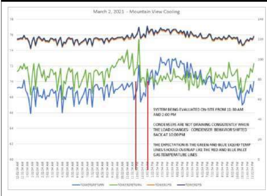
Figure 4. Condenser Drain Temperature Reversal. The green and blue lines are condenser drain leg temperatures. Readings are taken every 10 minutes. The top two lines are outlet drain leg gas pressure. Note that the green and blue lines swap temperatures in the early afternoon and then shift back at about 7:00 pm. It was during one of these reversals that the possibility of flooding back down the foul gas line became evident.
