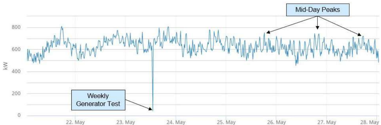
Figure 6. Cold storage facility interval data
