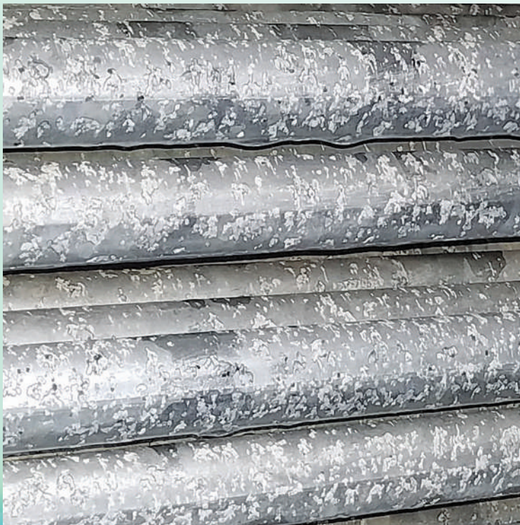
White Rusted Coil without Pass-Protect
